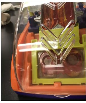
12. The lid will unlock when the heat tray and mold are cool enough to touch. The large knob will point to the unlocked icon. You can remove the green brackets from the machine and wait for 15 minutes for the wax to harden. The wax is very soft and fragile at this time
